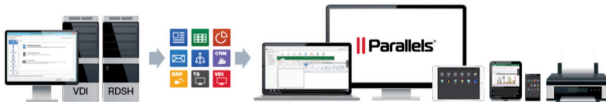
Figure 1. Parallels RAS: How applications and VDI are delivered to end users using Microsoft® Remote Desktop Session Host (RDSH)
